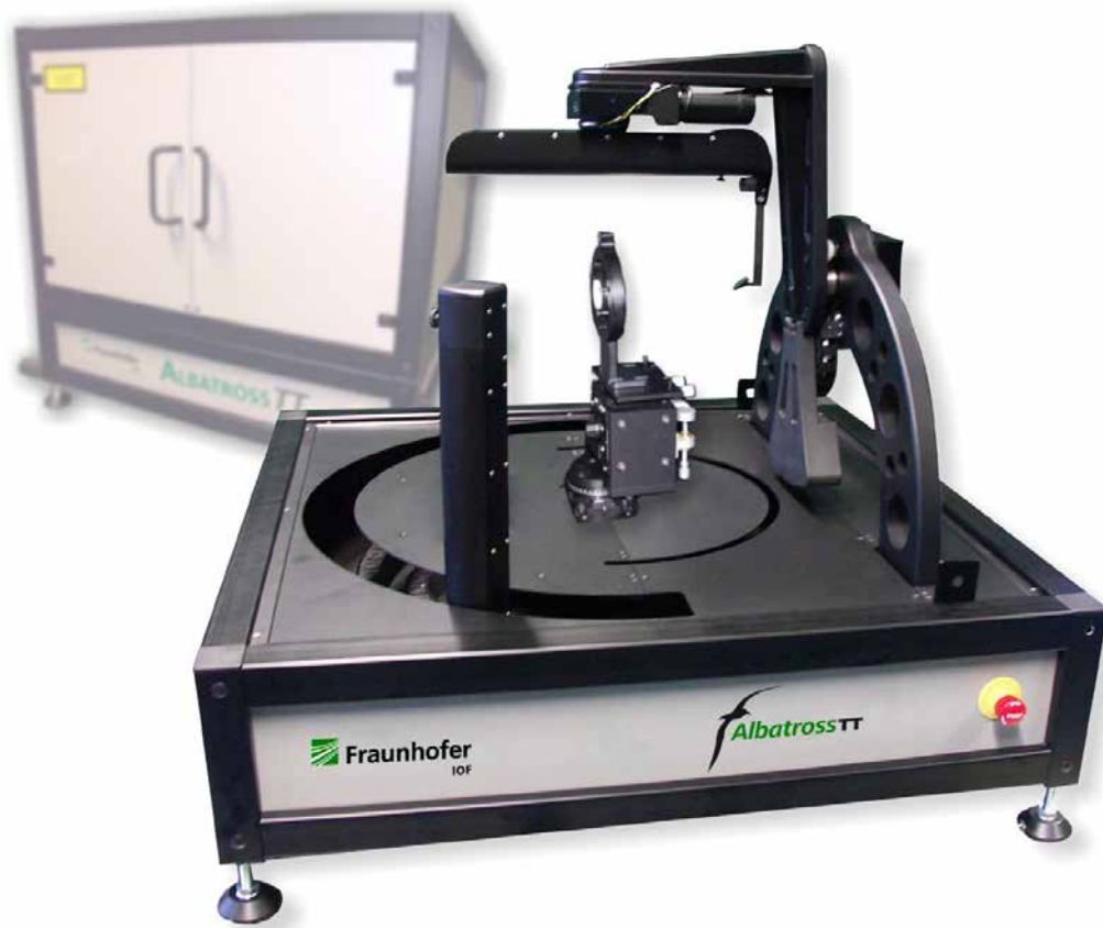
Light scattering measurement system Albatross-TT (Fraunhofer IOF)
